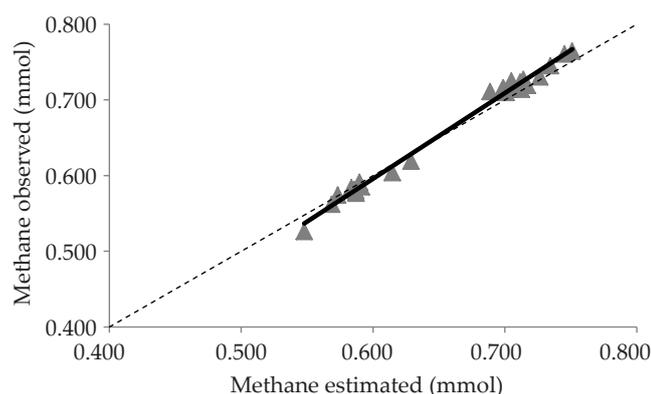
Figure 2. Plot between estimated (from volatile fatty acid profile) and observed (using infrared methane analyzer) methane emission. Regression equation: Methane observed =  $-0.084 + 1.133 \times$  Methane estimated ( $P < 0.001$ ;  $R^2 = 0.992$ ; RMSPE = 1.75%). Dashed line indicates an ideal line where the estimated methane emission is equal to the observed methane emission.
